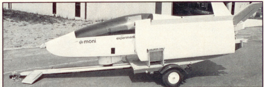
"One man, one airplane": All you need is $5,500 for the kit, sandpaper, paint, wood for the wing fixtures and about 400 hours building time. The Moni that results can be ground-handled solo, including assembly, disassembly and getting it on and off the circa-$400 Monnett trailer.
