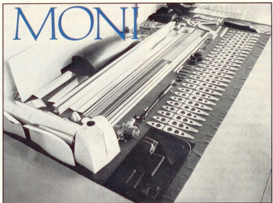
"One man, one airplane": All you need is $5,500 for the kit, sandpaper, paint, wood for the wing fixtures and about 400 hours building time. The Moni that results can be ground-handled solo, including assembly, disassembly and getting it on and off the circa-$400 Monnett trailer.
